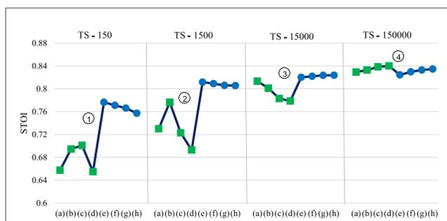
**FIGURE 8.** STOI score for (a) DDAE1, (b) DDAE2, (c) DDAE3, (d) DDAE4, (e) H-ELM1, (f) H-ELM2, (g) H-ELM3 and (h) H-ELM4, using different amounts of training batch samples (TS).
