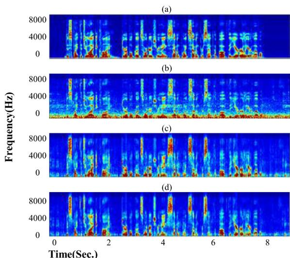
FIGURE 5. Spectrograms of an utterance (a) clean (PESQ = 4.6439), (b) noisy (PESQ = 2.2976), (c) ELM (PESQ = 2.3018), and (d) H-ELM (PESQ = 2.5489) contaminated with babble noise.
