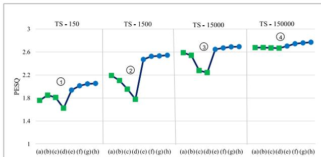
**FIGURE 7.** PESQ score for (a) DDAE1, (b) DDAE2, (c) DDAE3, (d) DDAE4, (e) H-ELM1, (f) H-ELM2, (g) H-ELM3 and (h) H-ELM4, using different amounts of training batch samples (TS).
