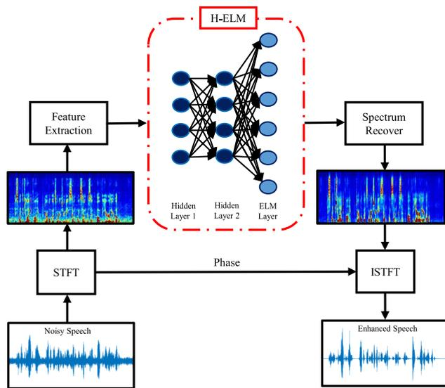
FIGURE 2. H-ELM-based speech enhancement architecture.
