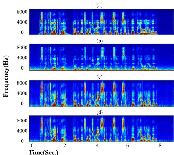
FIGURE 6. Spectrograms of an utterance (a) clean (PESQ = 4.6439), (b) noisy (PESQ = 2.4433), (c) ELM (PESQ = 2.5258), and (d) H-ELM (PESQ = 2.7345) contaminated with car noise.
