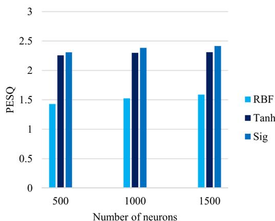
FIGURE 3. PESQ scores for ELM with different activation functions and numbers of hidden neurons.
